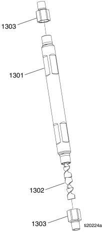
$\triangle$  Apply pipe sealant to all non-swiveling pipe threads.
